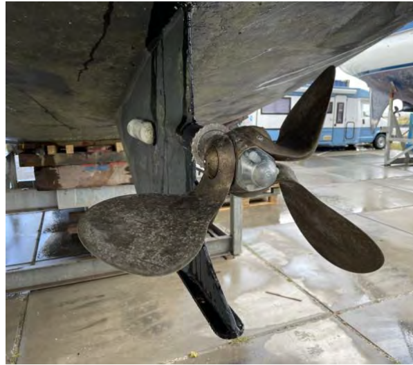
Folding prop Autoprop H6 with new bearings and anode
